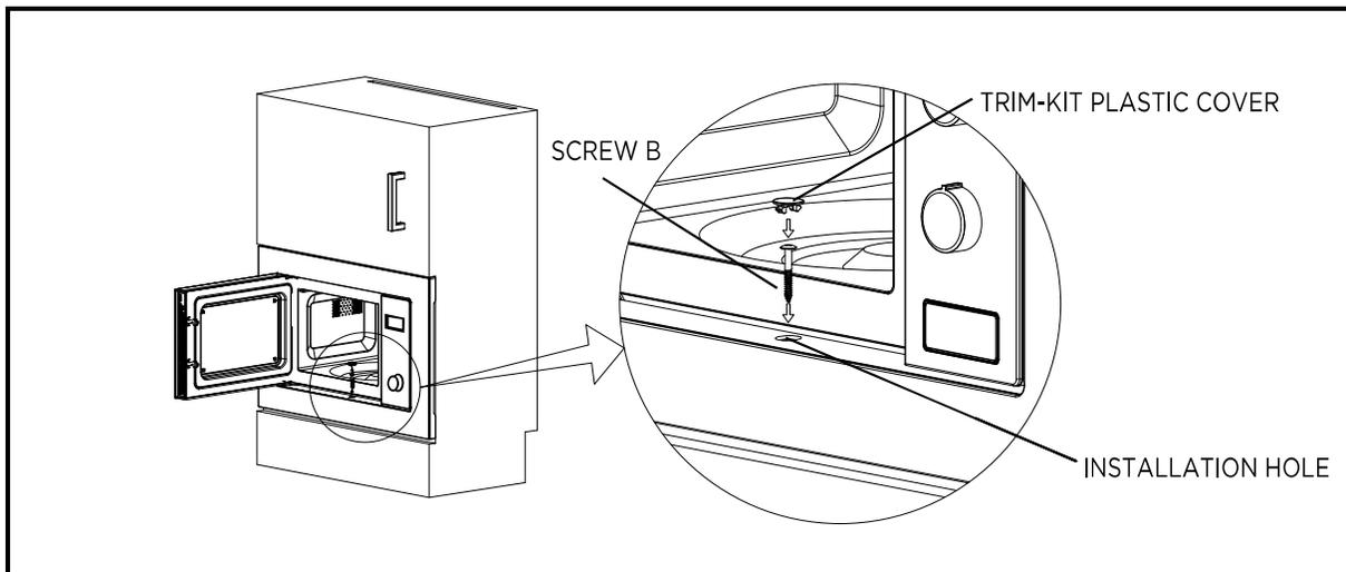
2. Open the door; fix the oven to the cabinet with SCREW B at the INSTALLATION HOLE of TRIM KIT. Then fix the TRIM-KIT PLASTIC COVER to the INSTALLATION HOLE.
