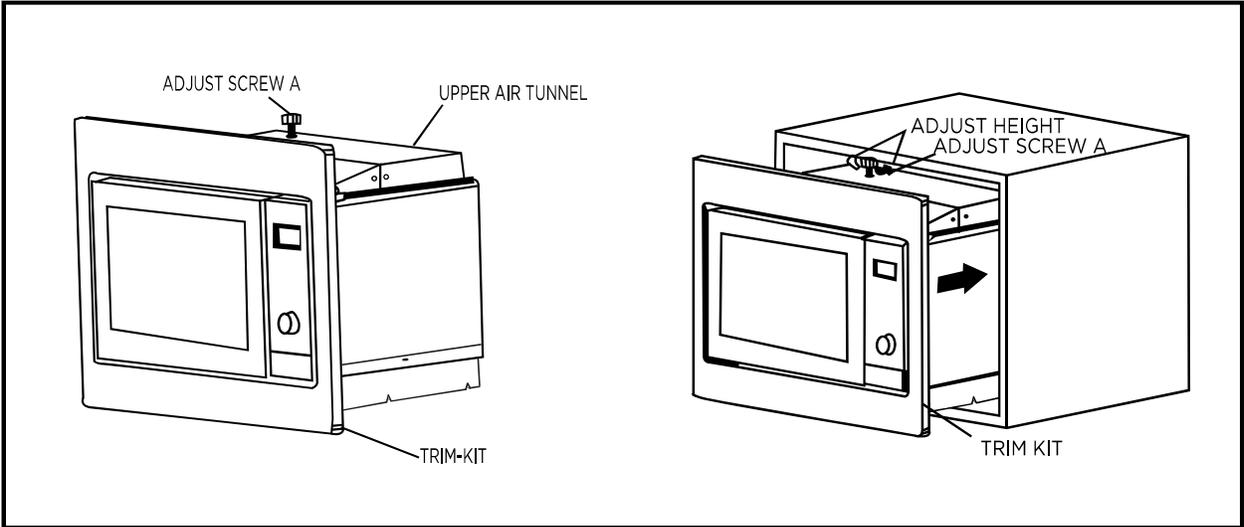
1. Fix ADJSUTSCREW A on the UPPER AIR TUNNEL of the oven, and then install the oven into the cabinet.
